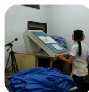
Measurement of sound level: Result 76 decibels meets standards
