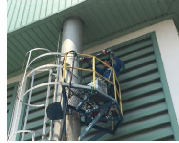
Check air quality from the vent (Stack Emission)
