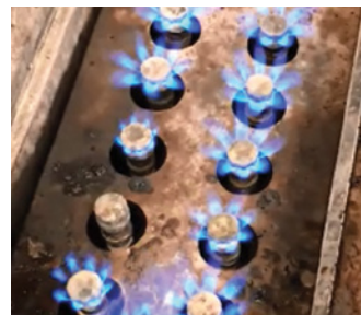
Gas Nozzle before Cleaning
