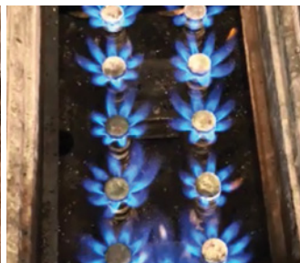
Gas Nozzle after Cleaning
