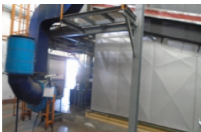
Picture #1 shows the measuring of an 8-hour average noise level measuring, within the Boiler Building
