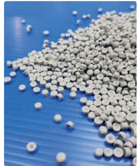
Specialty High-Density Polyethylene (HDPE) to Be Made into Floatation Devices for the Solar Farm
