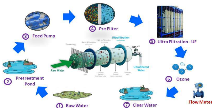
Water treatment process with ultrafiltration system and disinfection with ozone system
