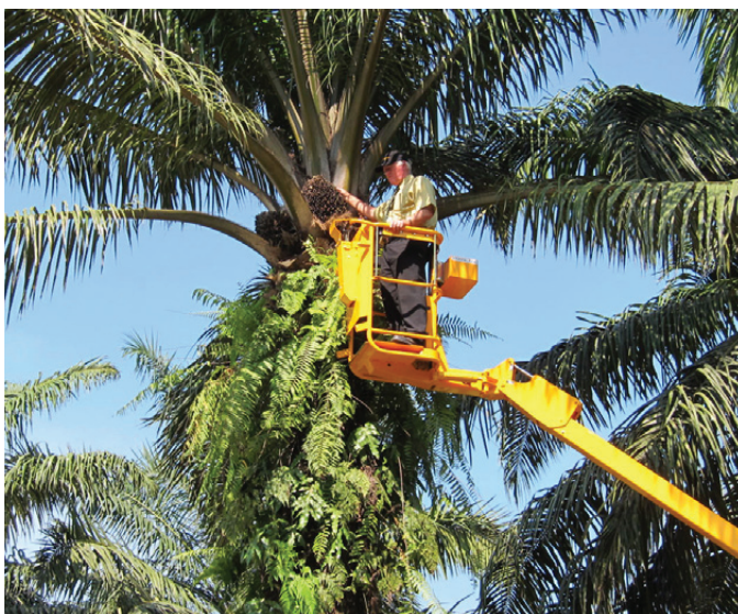
Hydralada work platforms are faster and safer than climbing ladders for seed garden operations
