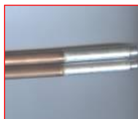
Aluminum welded with copper
