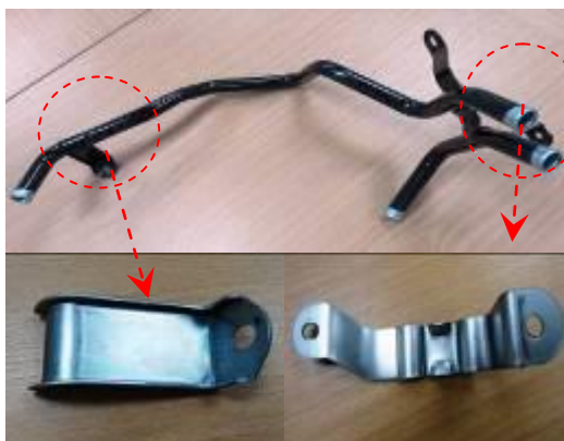
Pipe Water and Bracket
