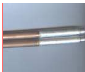
Aluminum welded with copper
