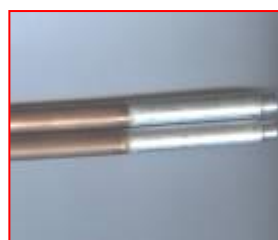
Aluminum welded with copper
