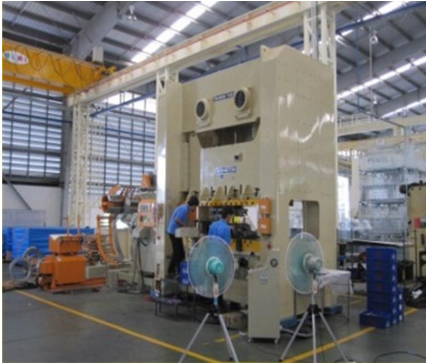
3.4 Tandem Line comprising of 300 ton press machines for 5 machines and 80 ton press machine for 2 machines
