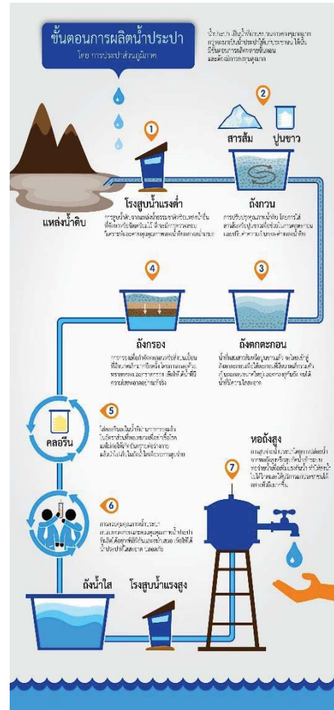
Diagram of Portable Water Plant Process (Source: Provincial Waterworks Authority)
