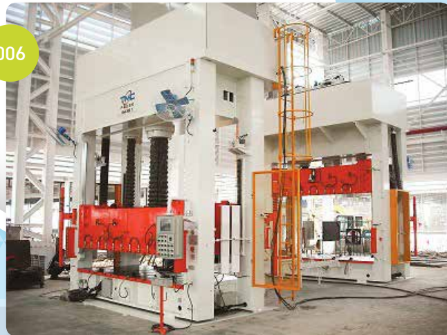
HHP: Hydraulic hemming spotting press
