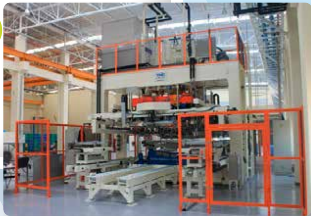
HSP: Hydraulic special forming press
