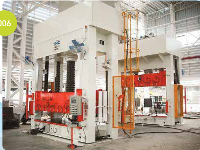
HHP: Hydraulic hemming spotting press
