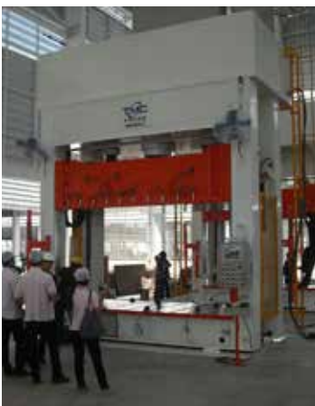
Hydraulic molding for hot press (HMP)
