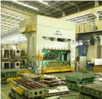
Hydraulic try out press (HRP)
