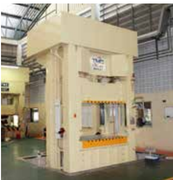
Hydraulic deep drawing press (HDP)
