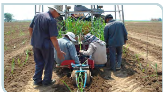
Demonstration of sugarcane planting by Shute Planter
