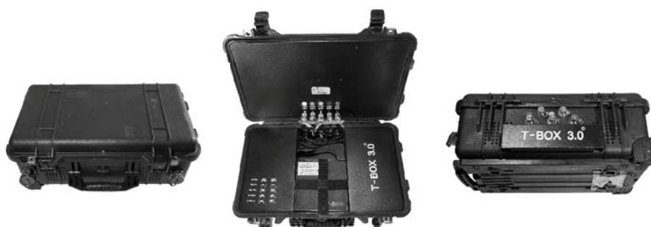
1.3 Radion Radio Audio Jammers, which were co-developed by PlanetComm and the National Electronics and Computer Technology Center (NECTEC) to block command signals from a mobile phone to other devices. The jammer is manufactured and sold exclusively to Thailand's government authorities responsible for maintaining national peace and security.
