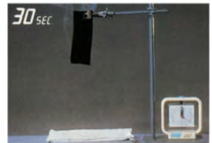
The Comparison of Burning demonstration of Tolyethylene Foam / Polyurethane Foam and Aeroflex EPDM insulation Rubber
