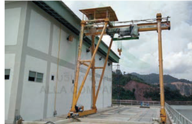
▲ Single Girder Gantry Crane
