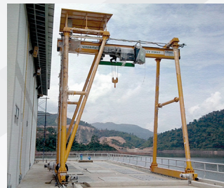
Single Girder Gantry Crane
