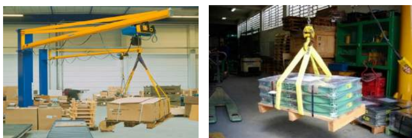
Sample images of using a webbing sling
