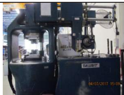
Sample image of a 2,000-ton crimping machine
