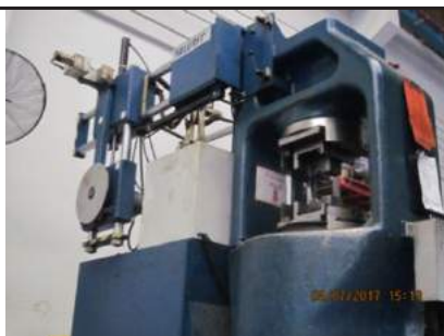
Sample image of a 2,000-ton crimping machine
