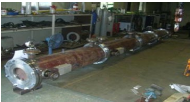
▲ Heat Pipe Fabrication
