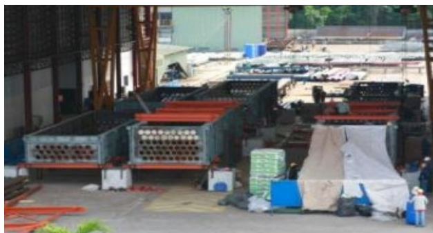
▲ Heat Exchanger Fabrication
