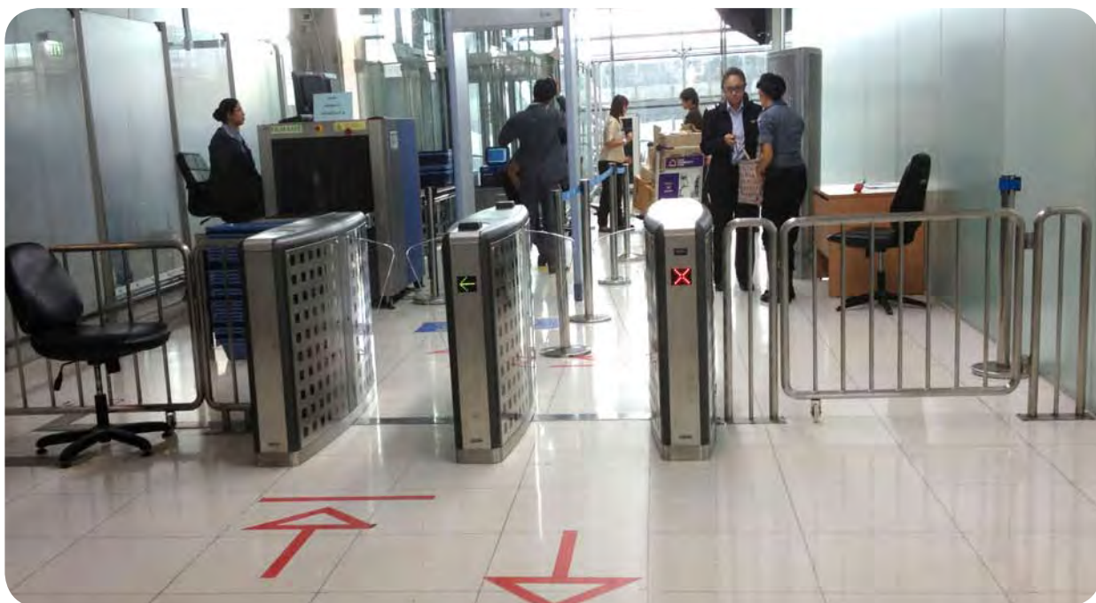
Control system for accessing airport restricted area where the personal security pass readers are installed.
