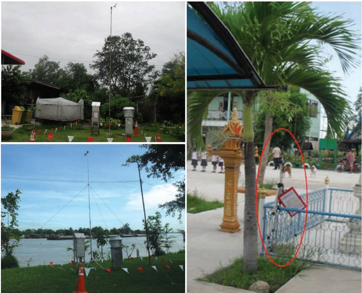
(left) Photographs of particle dust sampling and measurement for wind direction and speed at various locations (right) Photograph of noise level measurement
