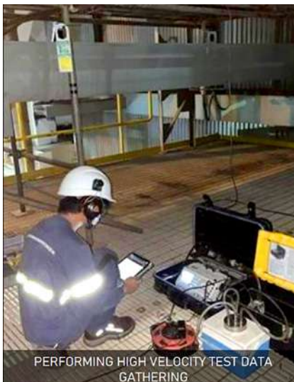
CONDUCTING AIR HEATER LEAKAGE TEST
