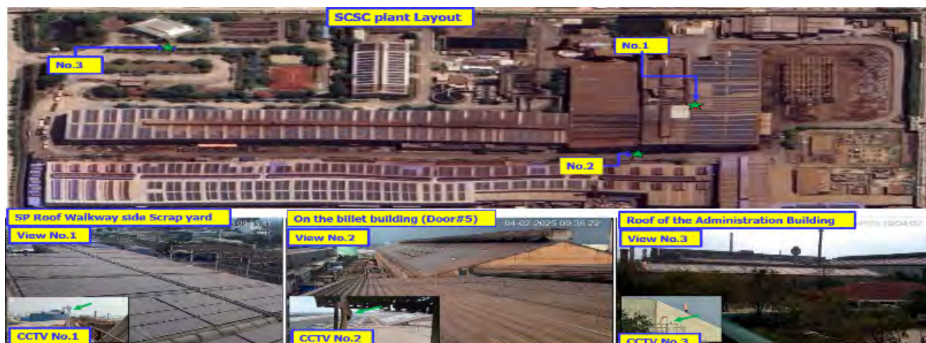
360° CCTV monitoring system and installation locations at SCSC plant for safety and environmental control
