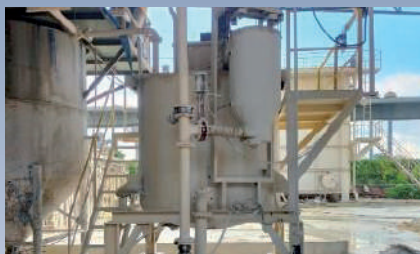
The wet sludge return system in the fiber cement tile production line reduces sludge across all production lines.
