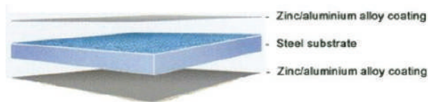
The image shows the coating layer of non-coated steel sheet.
