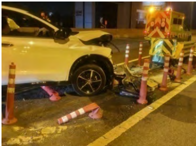
▲ Actions taken to reduce severity of accidents: installments of crash cushions and truck mounted attenuators
