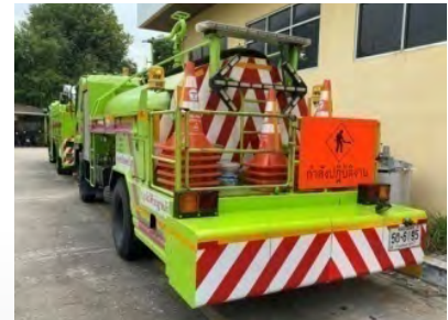
▲ Actions taken to reduce severity of accidents: installments of crash cushions and truck mounted attenuators
