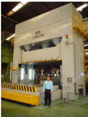
Hydraulic Try Out Press (HRP)
