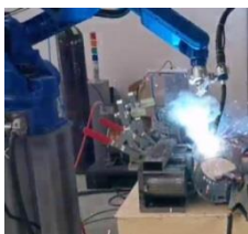
Picture of a robot installed in the motor parts welding production line.
