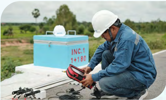
Dam Instrumentation (In-Place Inclinometer)
