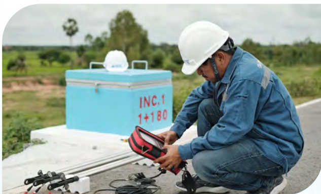
Dam Instrumentation (In-Place Inclinometer)
