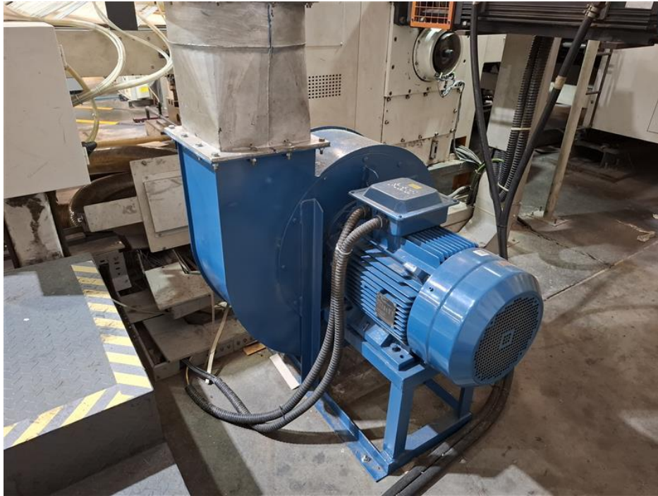
High-Efficiency Motor (IE4) Upgrade for Suction Fan Project: Bangkok Visypak Co., Ltd.
