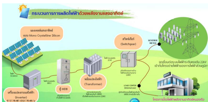
Example of the Electricity Generation Process of a Solar Power Plant Project
