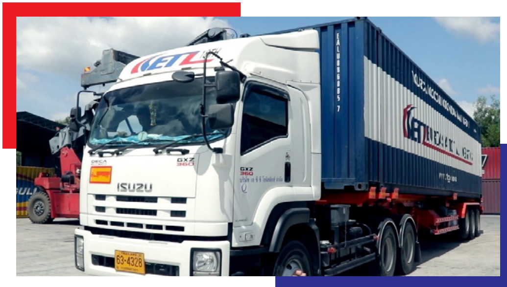
Prime Mover and Semi-trailer Carrying Standard Dry Containers
