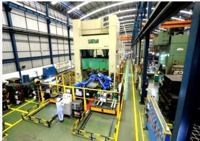
Tandem Line by Robot ขนาด 600 Tons
