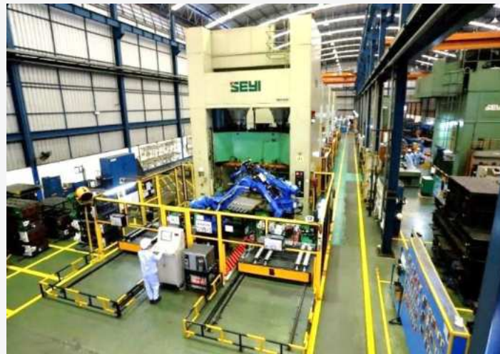
Tandem Line by Robot 600 Tons
