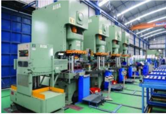
Tandem Press Line by Automatic Spacer
