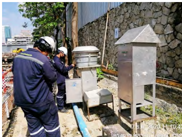
Monthly Dust Measurement to Ensure that Dust does not Exceed the Standard Value.
