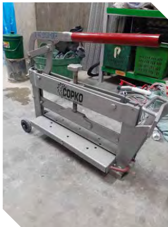
Aerated brick cutting machine is used to reduce dust and rubbles
