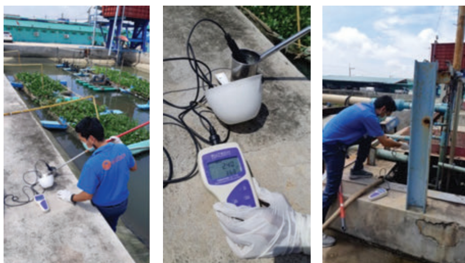
Image: testing and analyzing the quality of the released water by the authorized company
