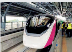
Train No.8 - Manual drive test from main workshop to Min Buri Station (PK30)
