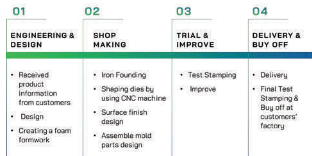
Stamping Dies Manufacturing Process Diagram
