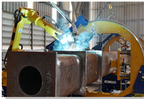
Picture of Robot welding machine
