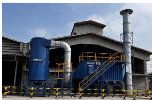
Install a solution deodorization system at the concrete tile production line
