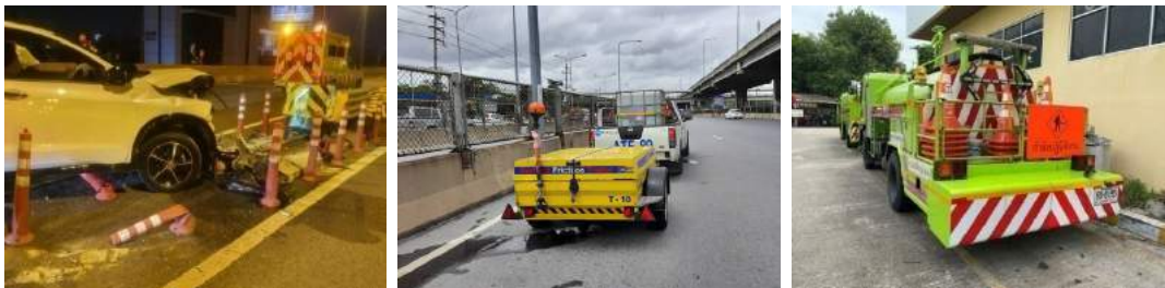
Actions taken to reduce severity of accidents: installments of crash cushions and truck mounted attenuators
