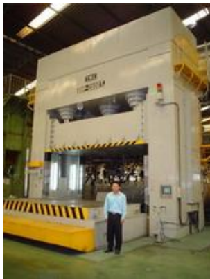
Hydraulic try out press (HRP)
