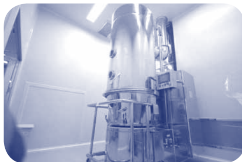
Drying using fluid bed dryer
