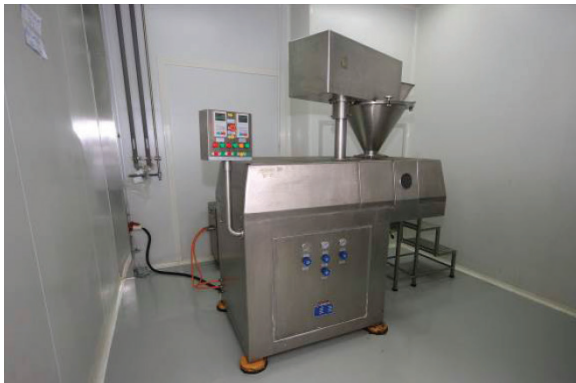
Dry granule rotary compression machine
