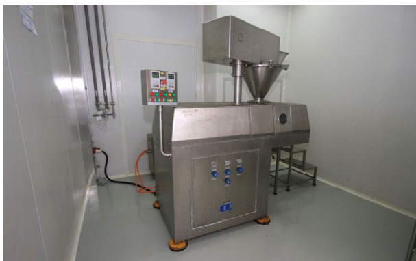
Dry granule rotary compression machine
