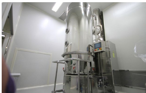
Drying using fluid bed dryer
